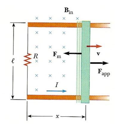
In the figure, we are applying a force this time to the rod. Due to Lenz's Law the magnetic force opposes the applied force. Since we know that the magnetic force acts to the left and the magnetic field acts into the page, we can use the RHR to determine the direction of the current around the loop and the resistor.
