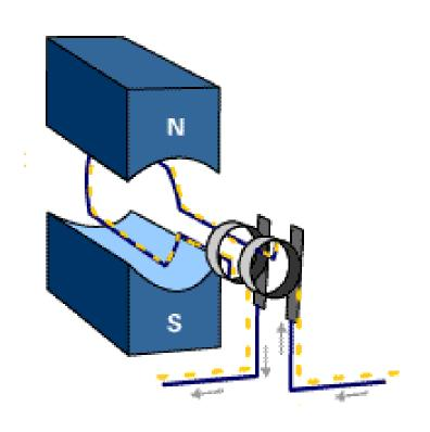
AC Generators use Faraday's law to produce rotation and thus convert electrical and magnetic energy into rotational kinetic energy. This idea can be used to run all kinds of motors. Since the current in the coil is AC, it is turning on and off thus creating a CHANGING magnetic field of its own. Its own magnetic field interferes with the shown magnetic field to produce rotation.
