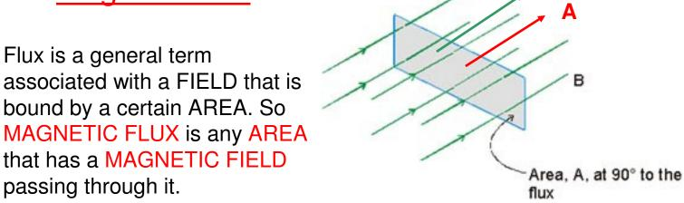
We generally define an AREA vector as one that is perpendicular to the surface of the material. Therefore, you can see in the figure that the AREA vector and the Magnetic Field vector are **PARALLEL**. This then produces a DOT PRODUCT between the 2 variables that then define flux.
