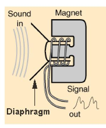
A microphone works when sound waves enter the filter of a microphone. Inside the filter, a diaphragm is vibrated by the sound waves which in turn moves a coil of wire wrapped around a magnet. The movement of the wire in the magnetic field induces a current in the wire. Thus sound waves can be turned into electronic signals and then amplified through a speaker.
