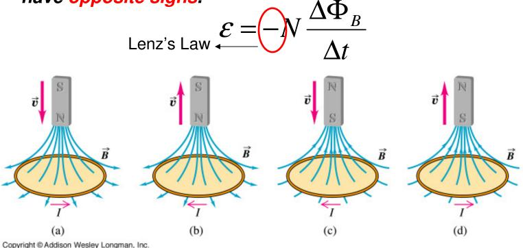
In the figure above, we see that the direction of the current changes. Lenz's Law helps us determine the **DIRECTION** of that current.
