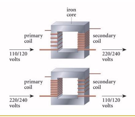
If the secondary coil has MORE turns than the primary you can step up the voltage and runs devices that would normally need MORE voltage than what you have coming in. We call this a STEP UP transformer.
