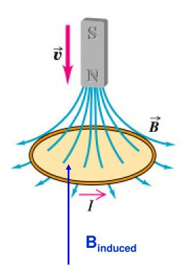
Let's consider a magnet with it's north pole moving TOWARDS a conducting loop.
