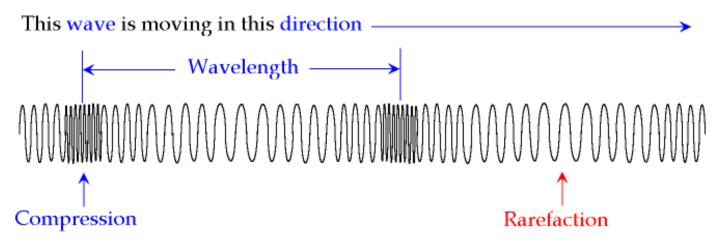
Longitudinal Wave - A fixed point will move parallel with the wave motion
