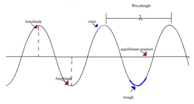
Transverse Wave - A fixed point will move perpendicular with the wave motion.
