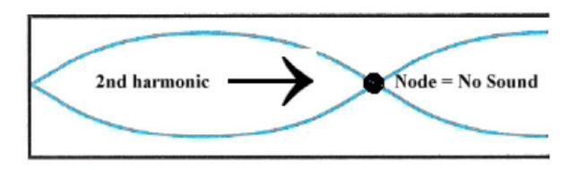
In a closed pipe, you have a NODE at the 2nd harmonic position, therefore NO SOUND is produced
